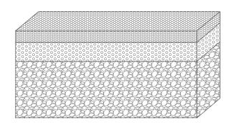
30mm thick 6mm aggregate wearing course 50mm thick 20mm aggregate base course
